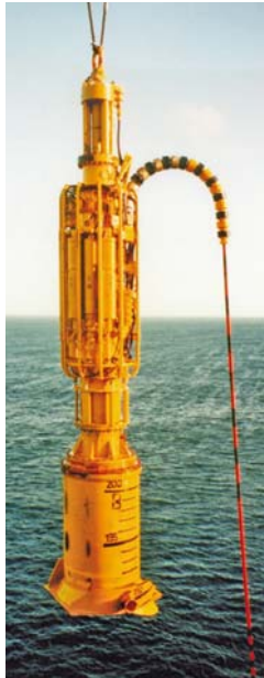
Sub-sea hammer for the off-shore platform installation require very robust control systems
