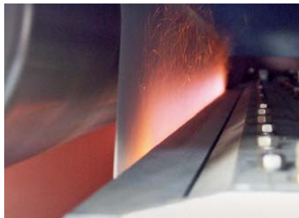
Figure 5: During singeing, very fine hairs and threads are removed from the fabric's surface
