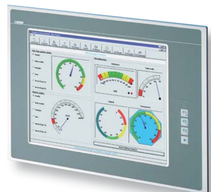
Figure 2: As a hardware platform, Osthoff-Senge uses Industrial-PCs from Lenze
