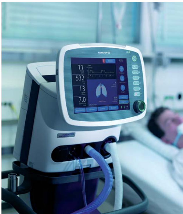
Respirator by Hamilton using an embedded CAN network
