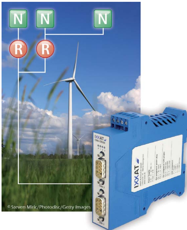
Figure 1: With CAN topology components, high bandwidths are possible even in extensive CAN networks
