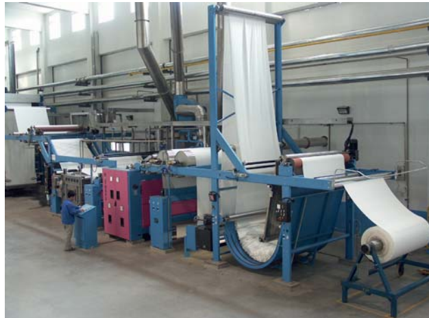
Figure 1: Textile finishing line with singeing station by Osthoff-Senge
