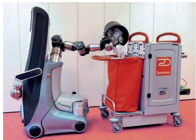
Figure 4: The lightweight arm is able to empty a full wastebasket
