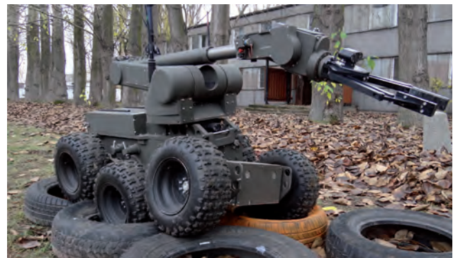
Figure 2: The Ibis is a six-wheeled robot for pyrotechnic and combat missions (Photo: PIAP institute)
