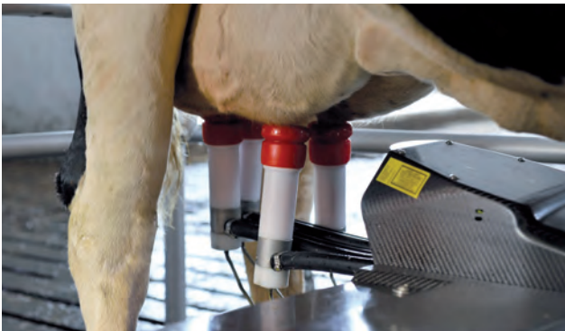
Figure 2: After going in the box the stainless-steel robotic arm moves under the cow, scans it with lasers to find the teats, and attaches four teat cups
