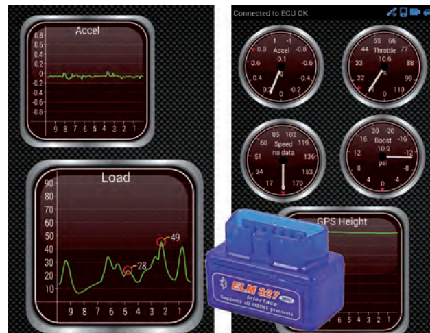
Figure 1: The ELM327 hardware interface and its available displays for data
