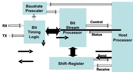
Figure 1. Basic architecture of CAN protocol controller
