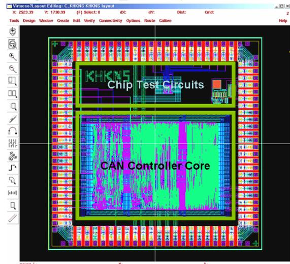
Figure 8. Layout of the designed chip
