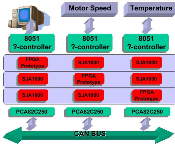
Figure 6. FPGA Verification System
