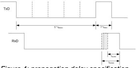
Figure 4: propagation delay specification for CAN FD transceiver
