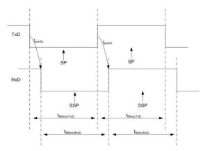
Figure 2: Transceiver with a perfect symmetric TxD to RxD propagation delay
