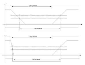
Figure 8: The impact of the transceiver internal bit time depends on the slew rate
