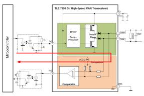
Figure 9: Optocoupler as interface for isolation
