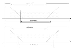
Figure 7: Comparison of TTL or CMOS transceiver TxD input concept
