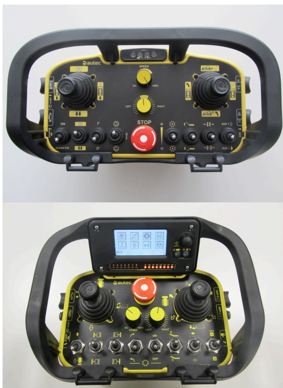
Figure 3: radio remote control for the mower, with and without display
