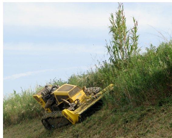
Figure 1: the mower working on a steep slope
