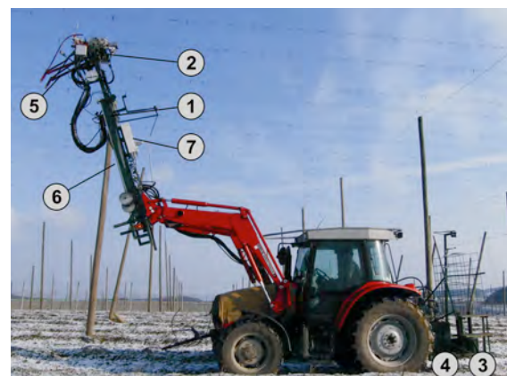
Figure 1: Prototype for automated attaching of the supporting strings in action during the testing in March 2013. Legend: (1) telescopic leader mast; (2)
