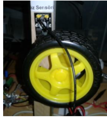
Figure 8: Wheel and Speed Sensor
