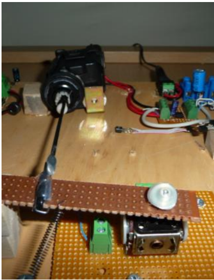
Figure 9: Servo-Mechanism and Throttle Position Sensor
