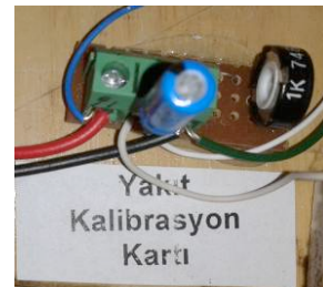
Figure 5: Fuel Level Signal Calibration Card
