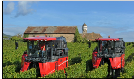
Figure 2: Automatic steering along the grape-vine rows
