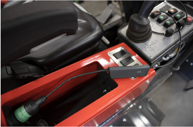
Figure 2: A dedicated J1939 diagnostics connector gives read-only access to the control system data, allowing live monitoring using TKE's CANtrace bus monitor tool (Source: Norcar, TK Engineering)
