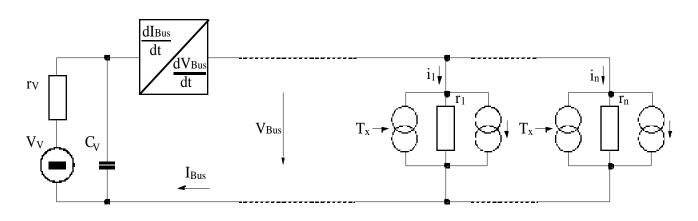
Figure 10: Current modulation
