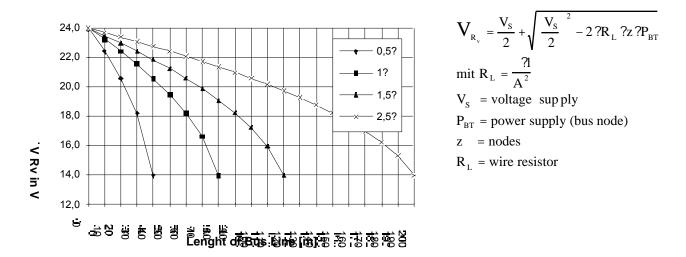
Diagram 1: Supply voltage by the last bus node (25 nodes a. 2 W power supply)
