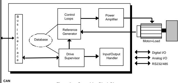
Figure 2 : Servodrive Block Diagram
