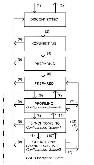
Figure 5. Bus Interface State Diagram
