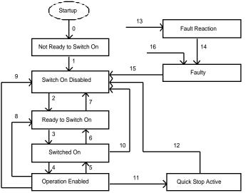
Figure 7. Drive Supervisor State Diagram
