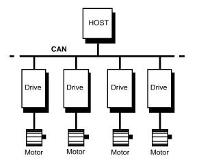
Figure 1. Block Diagram of CAN Servodrive System
