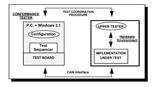
Figure 5 : Tester architecture
