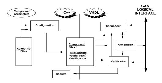
Figure 3 : CAN test plan architecture
