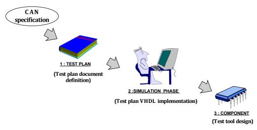
Figure 1 : CAN conformance testing methodology
