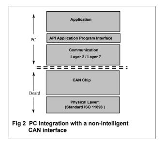
In applications involving non-intelligent interfaces, the communication software is processed on the PC. Due to the fewer number of components, these interfaces are less expensive, but have restrictions in processing networks having higher data transfer speeds and larger quantities of data. Before being applied, however, these cards must be checked whether suitable for the proposed application (see Fig. 3).
