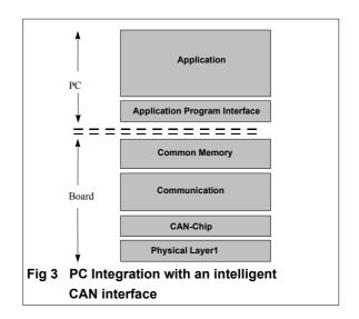
CAN interfaces are offered in all common formats. ISA and PCI interface formats are available for use in the PC. PC Cards in PCMCIA format type II (see Fig. 4) are specially available for mobile use, together with tools used in the configuration, integration, maintenance and service.
