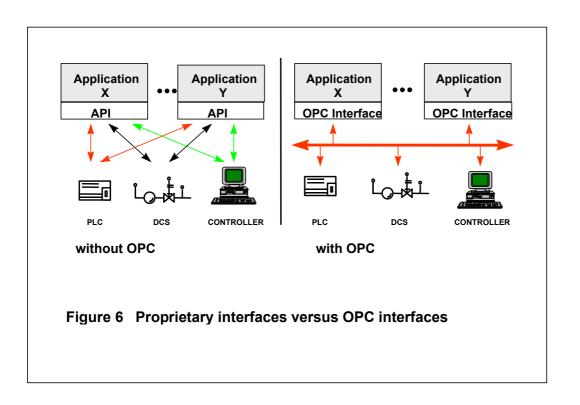
The integration of standards for CAN such as CANopen, DeviceNet<sup>TM</sup> and SDS with OPC leads to solutions compatible and interoperable to solutions of other OPC suppliers.
