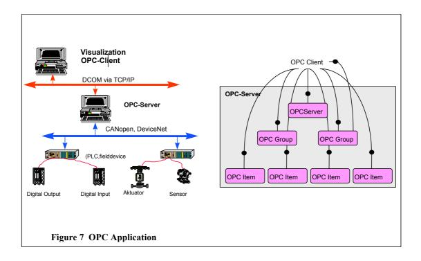
functionality as determined in the OPC specification. Parallel to this, an "Object" is also termed as OPC Server within the latter.
