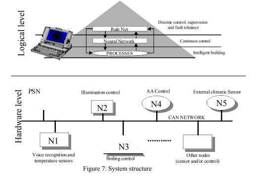
Physically, the system consists on at least six nodes, an PSN and five CN.
