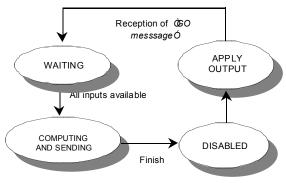
Figure 6: Output neuron state diagram
