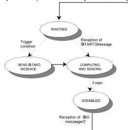
Figure 4: Input neuron state diagram
