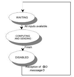
Figure 5: Intermediate neuron state diagram
