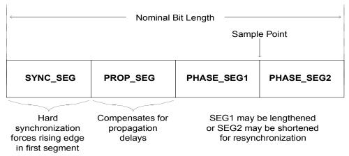
Figure 1. Partitioning of the Bit Timing Segments
