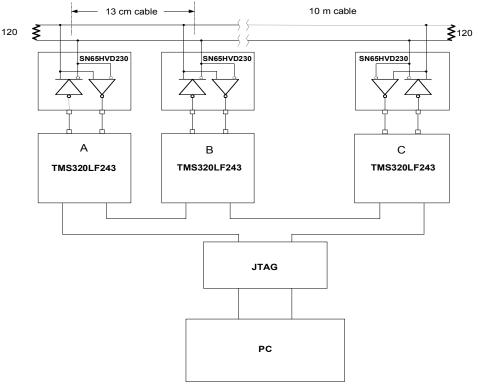
Figure 3. The Experimental 3-Node Bus
