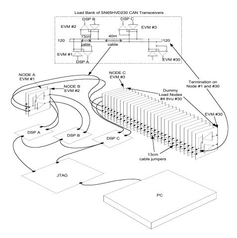
Figure 5. The 30-Node CAN Bus
