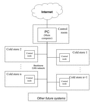
Figure 3. Hierarchy of networks and system architecture
