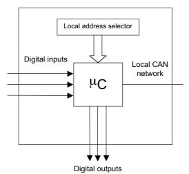
Figure 7. Digital I/O nodes structure
