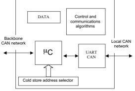
Figure 5. Central cold store nodes structure
