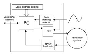
Figure 8. Ventilation control nodes structure
