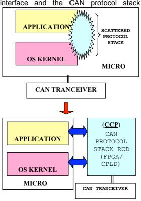
Figure 1: Migrating from the classical approach to the CAN co – processor approach.
