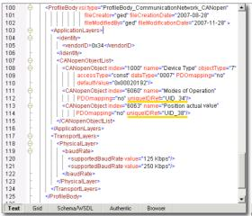
Figure 6: Part of CANopen object list with references to application process
