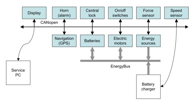
Fig.1: Possible system architecture in an LEV (e.g. Pedelec)
