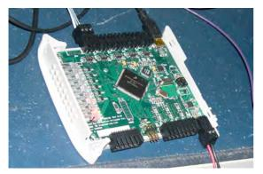
Photo 6 - New USB to 9S12 to 5x CAN "Assembled9S12-1.JPG"
