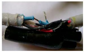
Photo 3 – Wire not Soldered "BadConnection.jpg"
