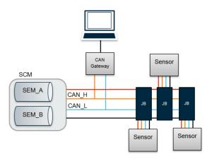
Figure 4: Subsea Control System Integration Setup
