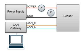
Figure 6: Power Consumption Setup
