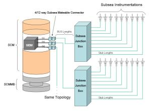
Figure 1: Typical Subsea CAN Topology
