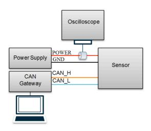
Figure 5: Inrush Current Setup
