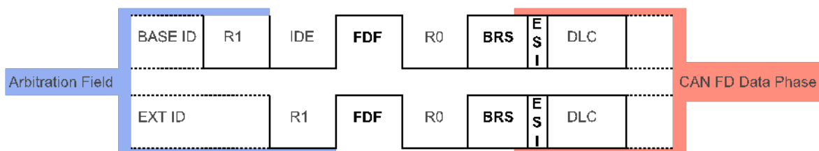
Figur 5: The bits that control the different CAN-FD functions
