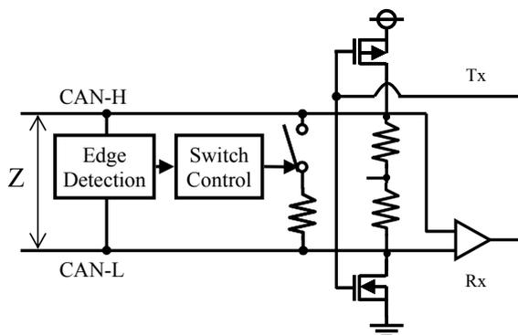
Figure 6 : Concept of ringing suppression circuitry
