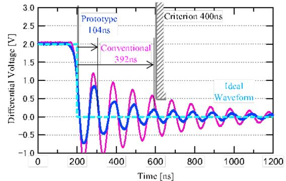
Figure 14 : Waveform on 4-ECU configuration (DLC3 bit)
