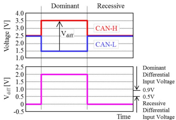
Figure 2: CAN FD typical voltage waveform
