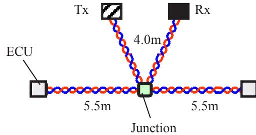
Figure 13 : Possible largest network using conventional CAN transceiver
