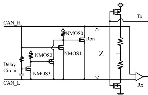
Figure 7 : Ringing suppression circuitry for explanatory example
