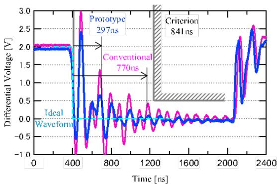
Figure 11 : Waveform on 8-ECU configuration (BRS bit)
