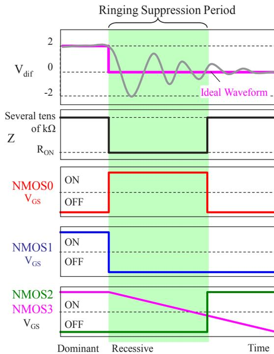
Figure 8 : Operating principle on proposed circuitry
