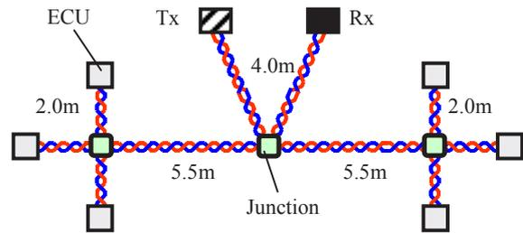
Figure 9 : Verification network configuration with 8 ECUs
