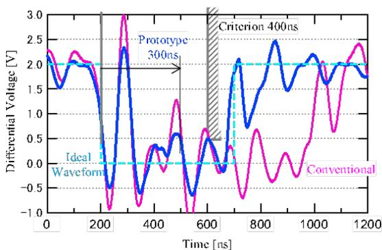
Figure 12 : Waveform on 8-ECU configuration (DLC3 bit)
