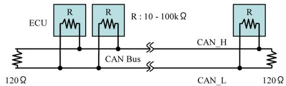
Figure 1: Physical layer of CAN FD
