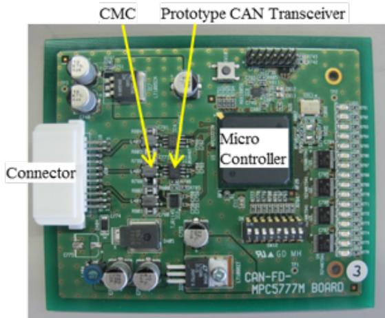
Figure 10 : Prototype CAN FD evaluation board
