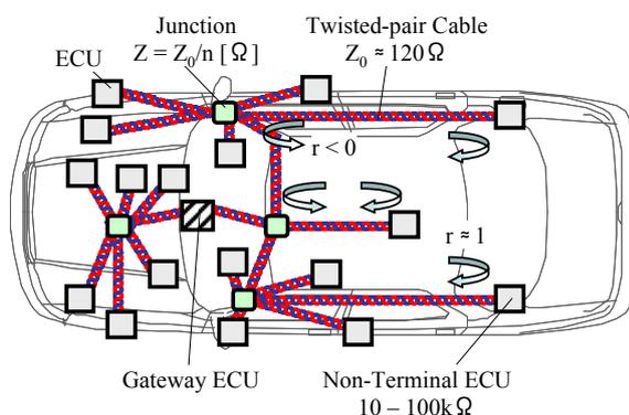
Figure 5 : Ringing generation mechanism
