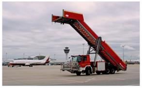
Figure 8: "Escape Stair" as a typical safety application
