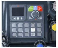
Figure 7: Operation via CAN key pane
