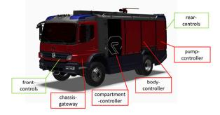
Figure 3: typical electronics distribution for municipal vehicle
