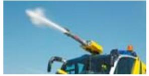
Figure 5: Water monitor 6,000 l/min
