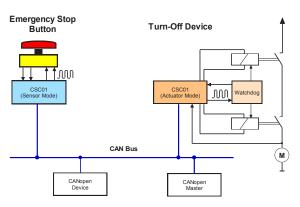
Figure 1: CANopen safety devices within a CANopen network
