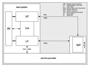
Figure 3: Local test method as defined in ISO 9646 1
