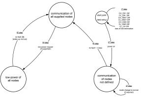
Figure 4: Example test flow
