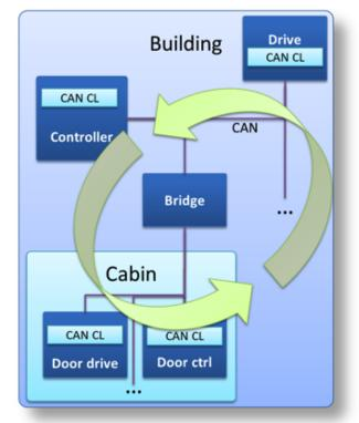
Figure 3: Using a CAN cryptographic layer, devices can be securely grouped and authenticate messages
