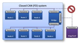
Figure 5: Temporary devices should not be allowed direct access to a CAN domain
