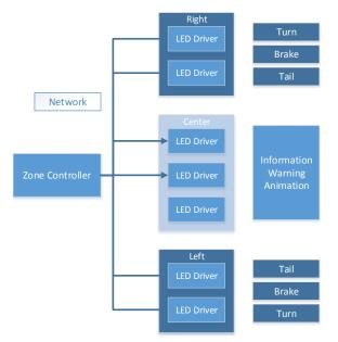
Figure 1 Rear Light Structure
